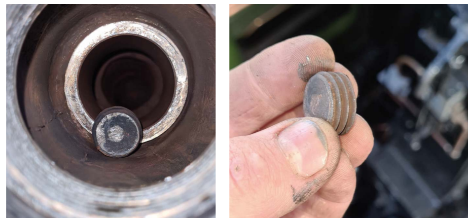
The foreign object found in the injector.
