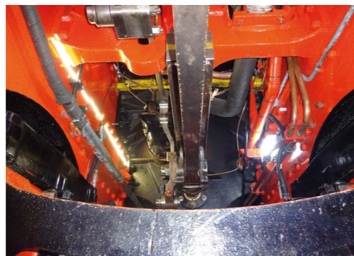
Above left: Rebuilt underframe lighting strips and bulkhead fitting beside the middle engine.
