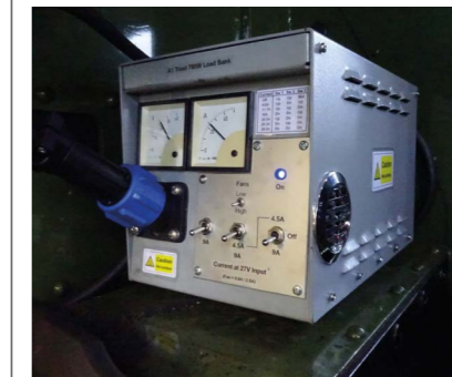
Above: Load Bank taking 24A from the ADA.
