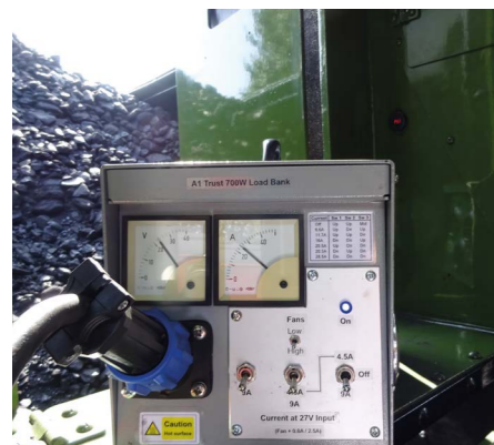
ETCS Load Bank taking 24A from the T2 turbogen supply.
